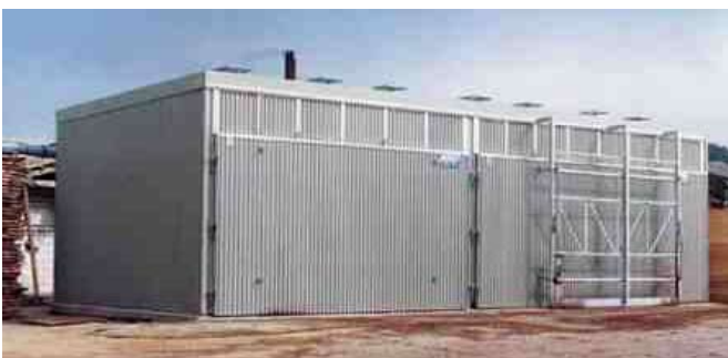
WOOD TREATMENT DRIER
